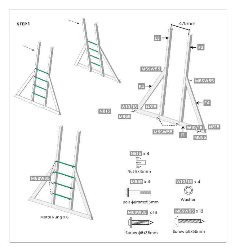
Try to ensure that the distance between the two support feet is parallel.
