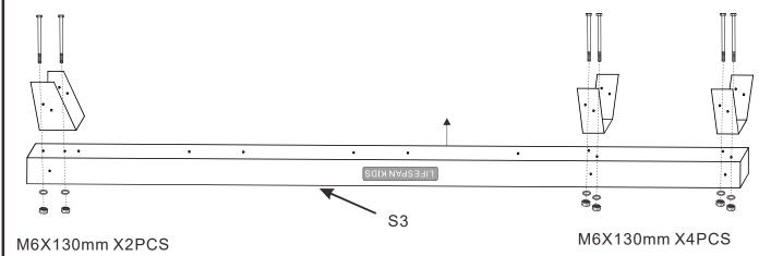
2.Build 6 spring hooks as per the figs and turn around beam to right direction for next step assembly..
