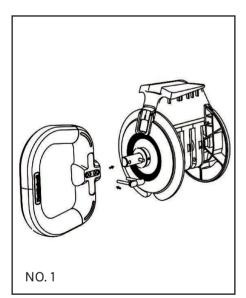
Install the adjusting handle and Kettlebell handle with bolts as shown.
