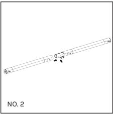
In the same way, install the other handle of the Barbell on the connecting rod by screws as shown.
