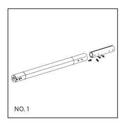
Install the handle of the Barbell on the connecting rod by screws as shown.
