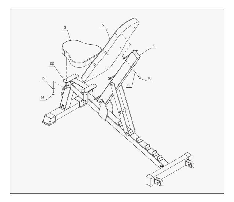
a. Secure 1 x Seat Pad (#2) to 1 x Seat Plate (#22) with:
