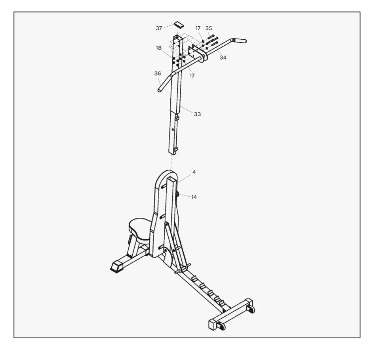
a. Secure 1 x Pull Up Tube (#33) to 1 x Support Frame (#4) with:
