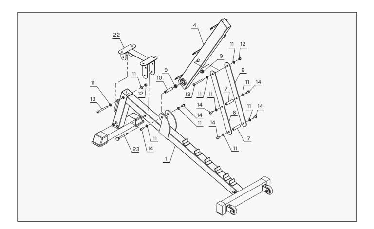
a. Attach the 1 x Seat Plate (#22) to 1 x Main Tube (#1) with:
