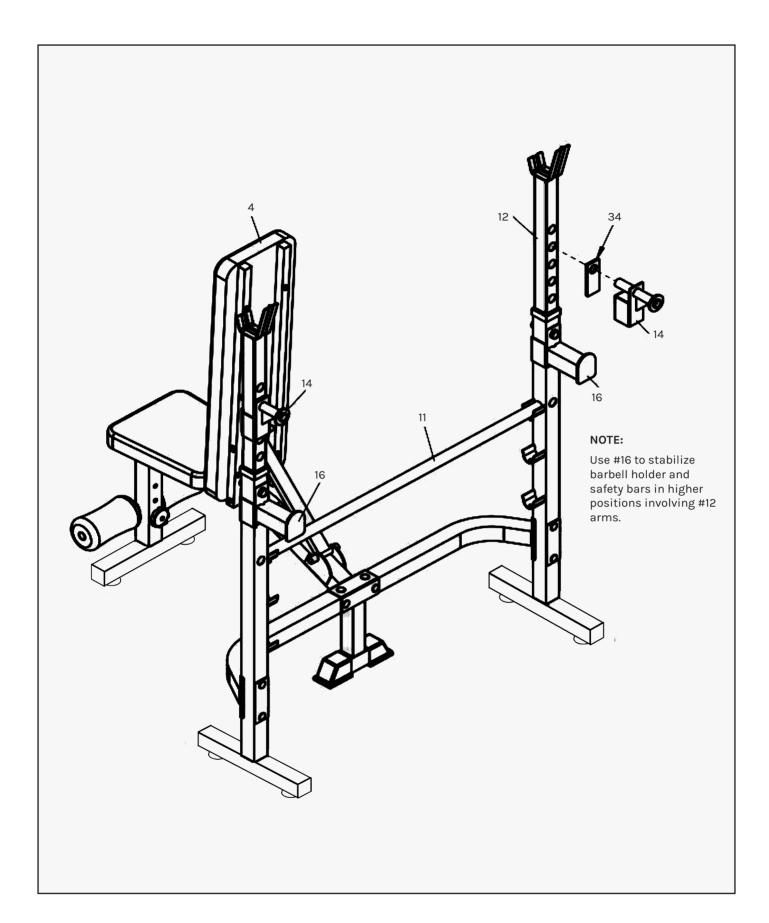
NOTE: When using the squat rack, please keep the Back cushion (#4) straight. Place both Bar J-hooks (#14) and (#16) into the 2x Support Tubes (#12) with 2x Plate (#34) in between. See above image. Part #34 is installed with #14 to act as a spacer.
