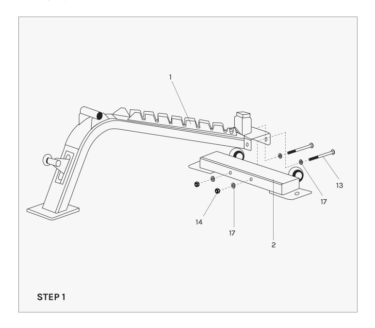
1. Attach Main frame (1) to The Bottom frame (2), using Screw M10X125 (13), Flat washer Φ10 (17) and Lock nut M10 (14).
