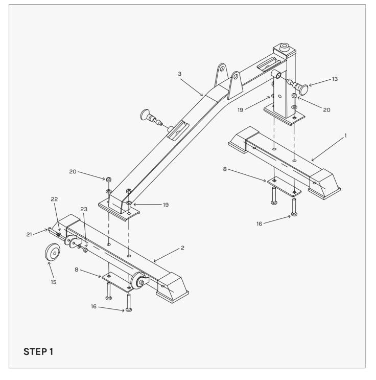
Use 16# (M10X70 carriage screw), 8# (connecting piece), 19# (Φ10 flat gasket), 20# (M10 anti-loosening mother) respectively to connect and fasten 3# (main frame) to 2# (rear sticking ground), 1# (front sticking ground), as shown. Then install 13# (pin welding) as shown in the two positions.
