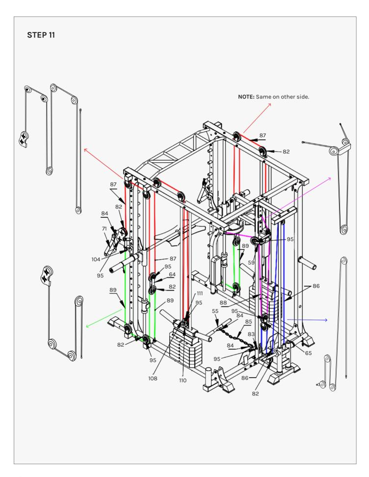
**NOTE:** Be sure to install the wire rope before installing the pulley.
