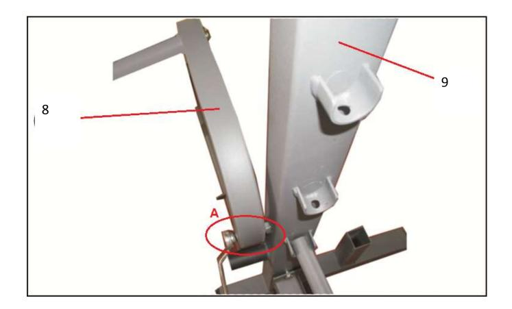
7. Bolt together the fly frame (8) and back frame (9) with 10mm bolts 120mm long (37) with washer (12) and nuts (34).
