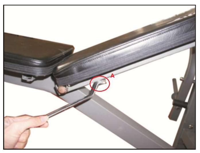
10. Using the 6mm bolt 35mm long (30) fasten the seated cushion (18) onto the main frame (12) . Fix the back cushion (19) to the main frame (17).
