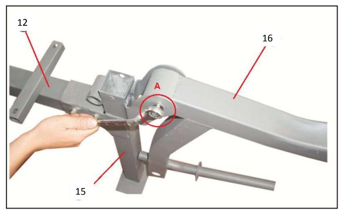
4. Bolt together fixed frame (16) and front fame (15) with 12mm bolts 75mm long (24) with washer (36) + nuts (33).
