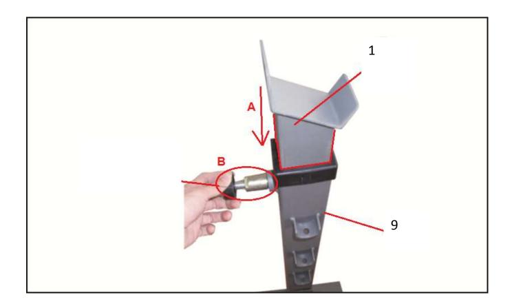
8. Insert adjustable frame (1) into the back frame (9) then fasten with pop pin.
