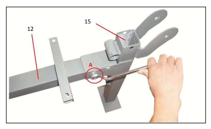
3. Bolt together main frame (12) and front frame (15) with 10mm bolts 65mm long (26) with washer (37) + nuts (34)
