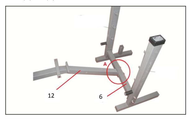
2. Bolt together the main frame (12) and cross beam (6) with 12mm bolts 75mm long (24) with washer (36) + nuts (33)
