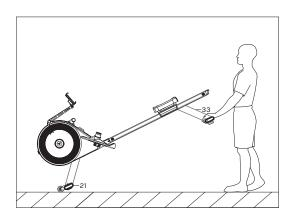
To move the machine, lift the rear stabilizer (33) until the transportation wheels (16) touch the ground. With the wheels on the ground, you can transport the machine to the desired location with ease.
