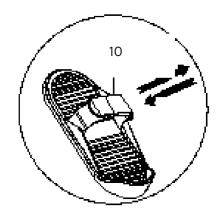
The pedal strap (10) is adjustable and can be personalized to fit the user's foot size.
