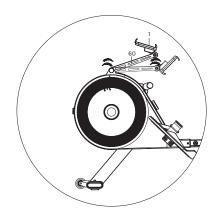
The rotation angle of Table holder (1) and computer post (60) can be adjusted to obtain the best view of the computer LCD screen.
