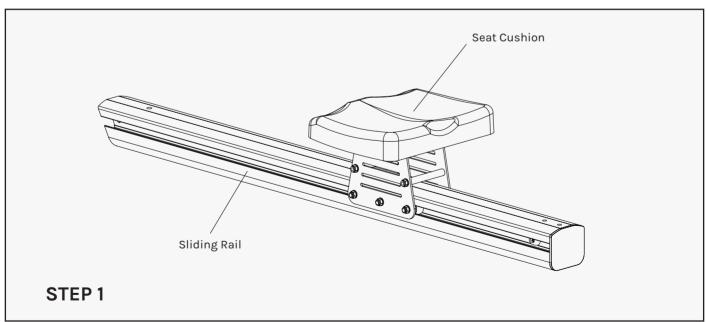
Remove the front stopper pad from the slide rail at the back, and then insert the seat cushion into the slide rail.
