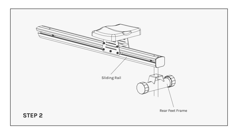
Connect rear feet frame to sliding rail with the 2 x M10\*50 bolt and nut.
