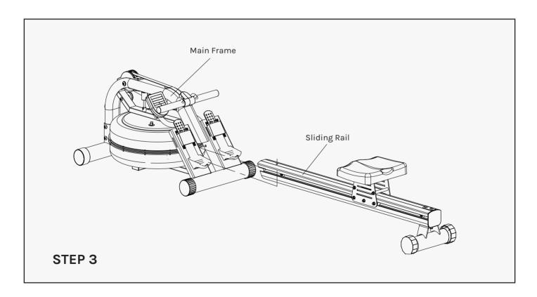
Lock up the sliding rail and main base frame with the screws.
