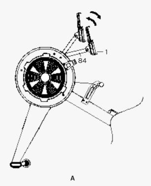
The rotation angle of computer post can be adjusted to obtain the best view of the console LCD screen.
