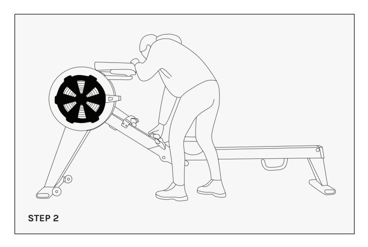
Then using the handle on Main frame (7), pull the rail up until you hear a click. Be careful of your fingers as the seat may roll back.
