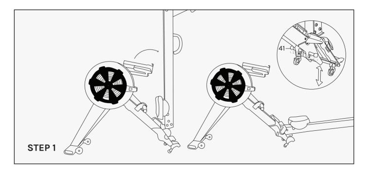
Hold onto the rail part and push the Adjusting spindle (41) down as pictured in image. You can then lower the rail down.
