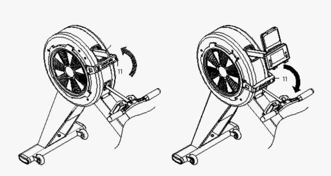
The rotation angle of air adjustable handlebar (11) can be adjusted to control air intake.
