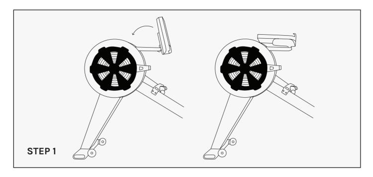
First rotate the display so it is moved out of the way.
