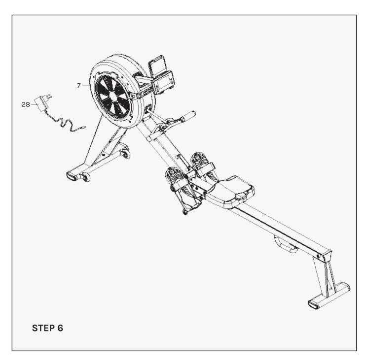
Insert the adapter line (28) to power hole on the back of main frame (7), then plug the adapter into an outlet.
