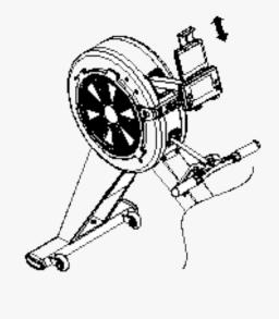
The width of iPad holder can be adjusted to different size tablet.
