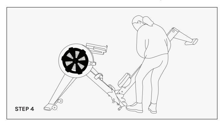
Pull the rail up from the back up into a vertical position. You will hear a click when it is locked in place.
