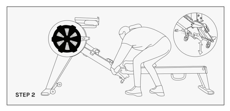
Pull the Adjusting spindle (41) up as pictured in image. It will drop down onto the wheels. Keep feet clear of the wheels.
