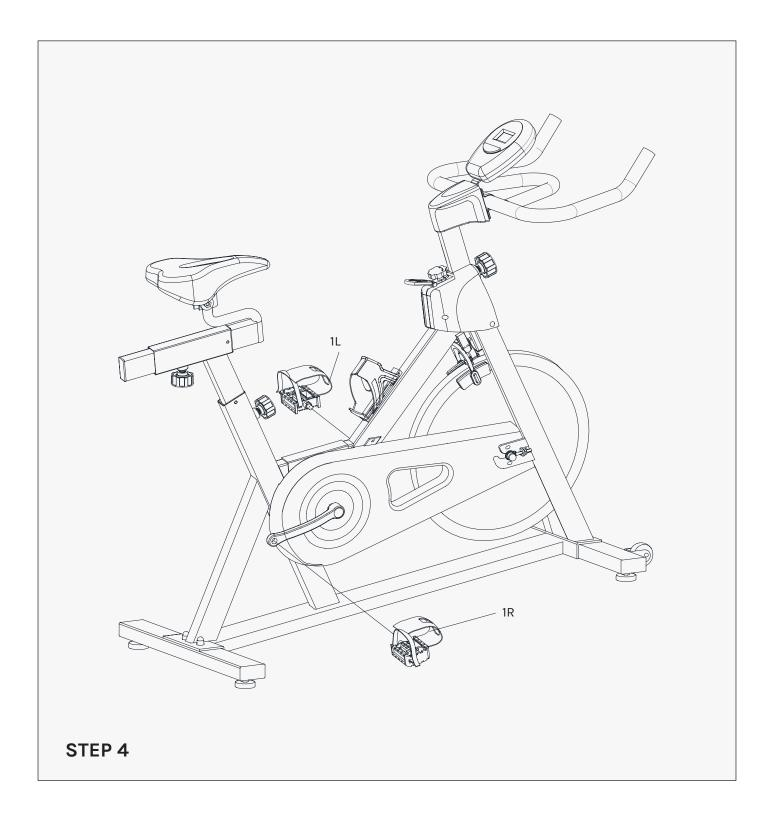
1. The Pedals (pt.1L & pt.1R) are marked "L" and "R" - Left and Right. Connect them to their appropriate crank arms. The right crank arm is on the right - hand side of the cycle as you sit on it.
