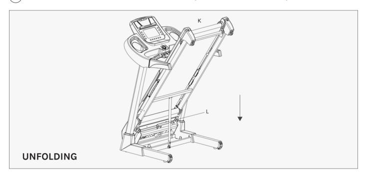
Grasp the Main Frame with one hand (position K) and use your foot to lightly kick the Air Pressure Cylinder (BO3) to unlock. Give the Main Frame a downward push from position K and the running deck should automatically continue to steadily lower itself until the Main Frame reaches level ground.
