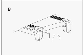
If the belt has drifted to the right: Whilst the treadmill is running at 4km/h, carefully turn the right adjusting bolt 1/4 turn clockwise. Then monitor treadmill until the belt centers. Repeat until the belt correctly centers.
