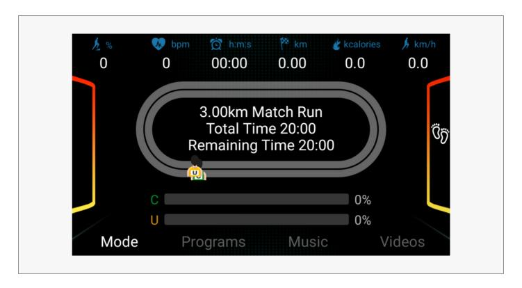
After choosing distance, press the "INCLINE"+/- or "SPEED" +/- buttons to adjust the match time. Press the START button to start.
