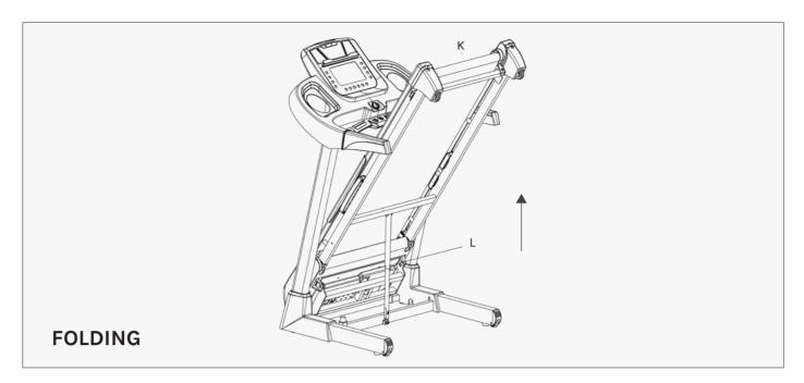
Place your hand at the end of the running deck (position K) and lift up the Main Frame until the Air Pressure Cylinder (B03) locks.
