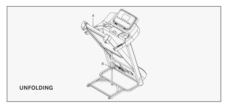
Whilst supporting position (A) with our hand, gently push position (B), the marked area on the air pressure bar, with your foot. The base frame will descend automatically. (Please keep people and any pets away the machine during descent)
