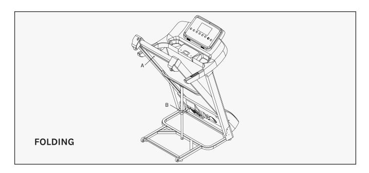
Place your hand on position (A), then pull up the base frame until you hear the click sound emitted when the air pressure bar (B) is locked into the round tube.
