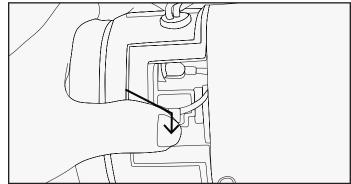
9a. Release the clip back into its position.
