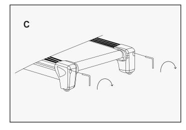
To adjust the tightness of the belt: Turn the treadmill off. Turn both the left and right adjusting bolts 1/4 turn clockwise. Repeat until the belt correctly tightens.
