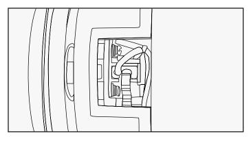
10. Check that the motor brush is held firmly in place by the clip, and that the lead is plugged securely onto the terminal.
