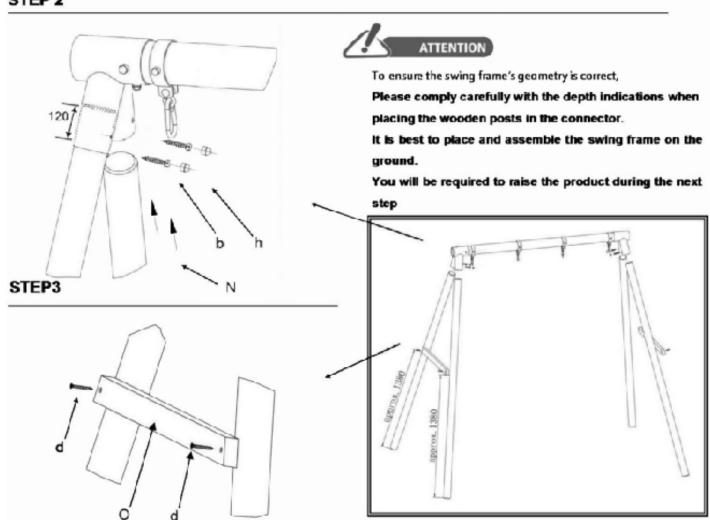
Note: the swing can be anchored directly into the ground using the anchors provided. You may also use cement for additional stability, please follow the below instructions.
