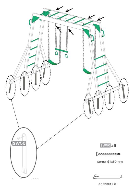
Install anchors as pictured with 2x on the inside middle section and 2x on the outside corners.
