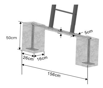
Dig holes for the underground anchor as per the size below. Please fill the hole with gravel or soil and compact properly before using.
