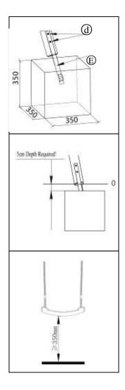
The distance from the ground to the swing element should be  $\ge$ 350mm
