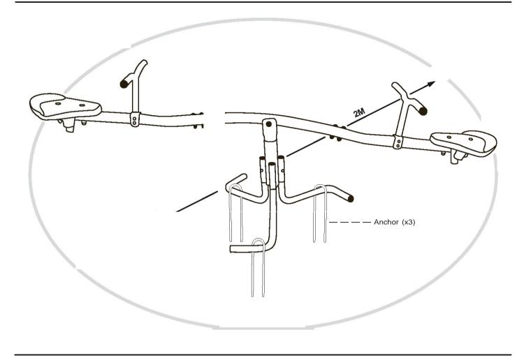
Now go back and tighten all screws firmly and check the spring-loaded joints
