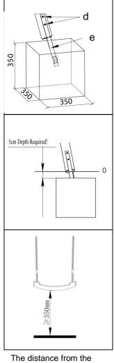
The distance from the ground to the swing element should be ≥350mm
