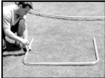
7 Connect both extensions to U-shaped piece as shown. Align the set-screws holes, insert large set-screws & tighten.
