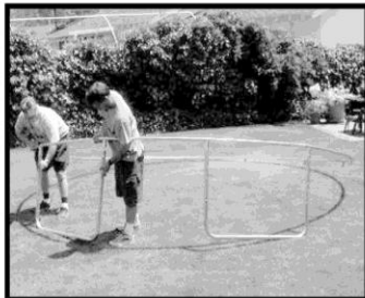
10 Repeat procedure for each U-leg and attach to top-rail with large set-screws.
