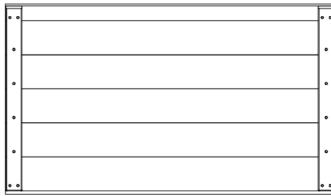
(1) RP1 - ROOF PANEL - W104046 1 3/8"x28 1/8"x48 3/4" (34x715x1238)
