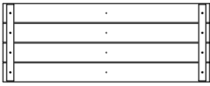
(4) FP1 - BOTTOM FLOOR PANEL - W2A01485 1 5/8"x13 1/2"x35 3/8" (40x344x897)
