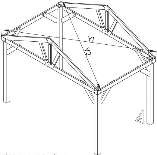
Check the frame measurements are same by measuring from one post to the opposite post diagonally and also the angles of the legs are at 90 degree angles.
