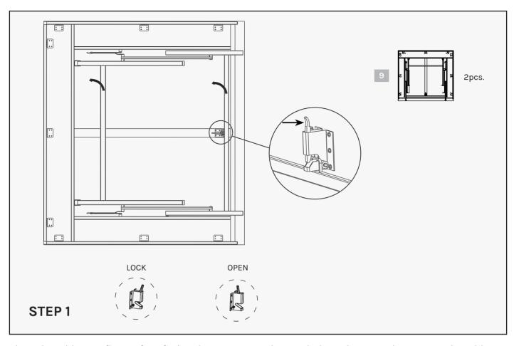
Place the table on a flat surface facing down. You can place a cloth on the ground to protect the table. Unlock the legs from the table. Then unfold the legs.
