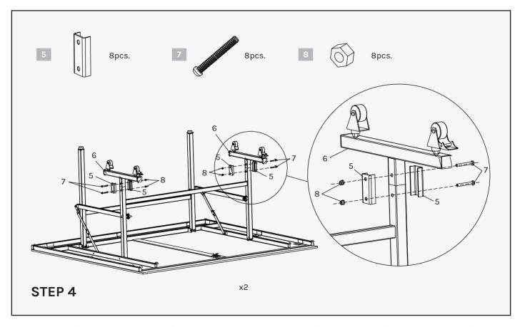
When attaching the Part 6 to the frame, ensure that both part 2 is on the outside and the part 3 is facing the frame leg as shown.
