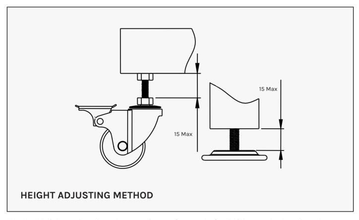
The wheel height can be adjusted to a maximum of 15mm. The foot height can also be adjusted to a maximum of 15mm.
