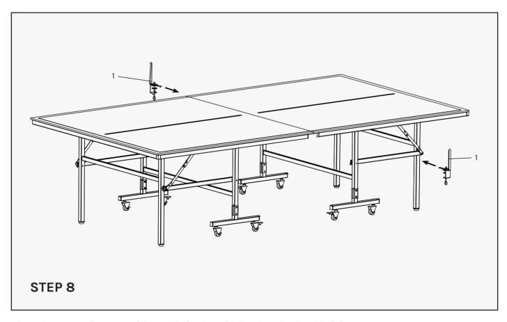
Place the part 1 pieces on either ends in the middle where both table joins.
