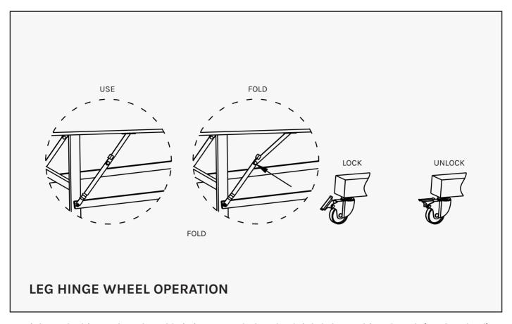
Straighten the hinge when the table is in use. Lock the wheel tightly by pushing the tab (on the wheel) down and lift up to unlock when you are transporting.
