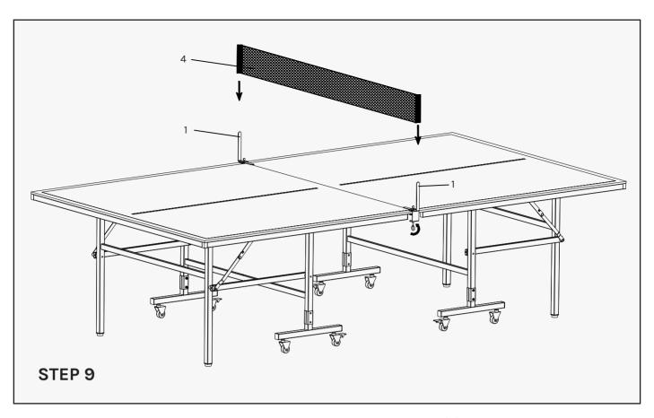
Turn the bottom fastening on part 1 to secure to table. Place the netting (4) to the part 1 bracket.
