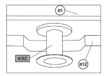
15. Firmly tighten all nuts & bolts on the leg assembly which were left only hand-tightened in Step 4. See diagram below:
