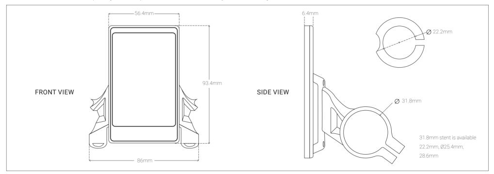
Outer shell material is ABS, Liquid crystal transparent window material is high hardness acrylic.
