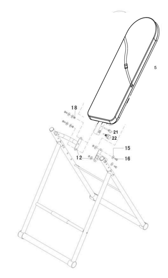
Use 4x Hex screw (16), 4x Washer (15) and 4x Nut (18) to secure part (5) to part (12).
