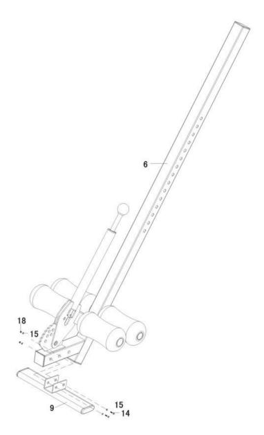
a. Secure part (6) to Foot Plate (9) with 2x Hex screw (14), 4x Washer (15) and 2x Nut (18).
