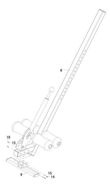
a. Secure part (6) to Foot Plate (9) with 2x Hex screw (14), 4x Washer (15) and 2x Nut (18).
