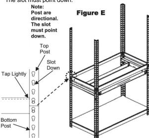
10. One rivet from each beam and brace must be placed in the top slot hole of the bottom post, and the bottom slot hole of the top post. After all beams and braces are in place, tap lightly to properly seat the rivets.
