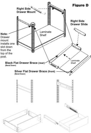
Assemble the top post to the bottom post by using two beams and two braces. Note: Posts are directional. The slot must point down.
