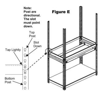
10. One rivet from each beam and brace must be placed in the top slot hole of the bottom post, and the bottom slot hole of the top post. After all beams and braces are in place, tap lightly to properly seat the rivets.
