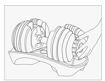
2. To properly select a desired weight, both adjustment knobs should be rotated so that the desired weight is aligned with the arrow in the middle. Then simply pull the handle straight up, this will remove the handle and the selected weight plates from the base.
