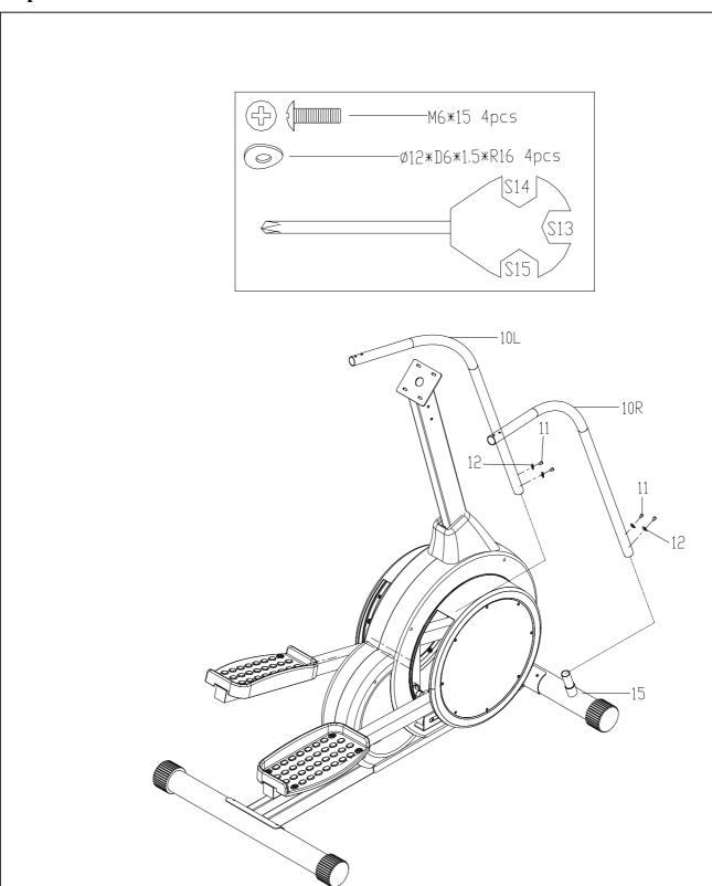
Lock middle handlebar (10L/R) to front bottom tube (15) with bolt (11), washer (12)., but do not tighten too closely;
