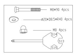
Lock front bottom tube (15) and rear bottom tube (25) to main frame (22) with bolt (17), washer (18), and nut (9).
