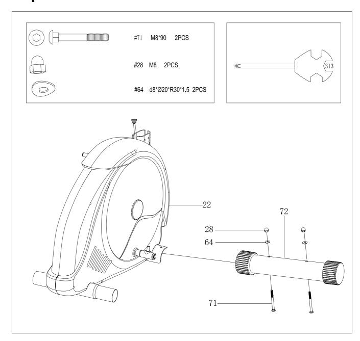
a. Secure the front stabilizer (72) to the main frame (22) by using square bolt(71), nut (28) and Arc washer (64).
