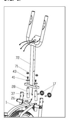
Connect the Wires (26 & 37) ,Then insert the
