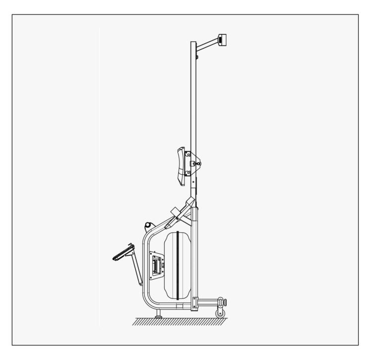
As shown above, when the product is not in use, the machine can be put upright to avoid taking up space as shown above.
