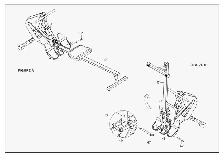
When not in use, you can save space by folding the Sliding Rail (No. 17).
