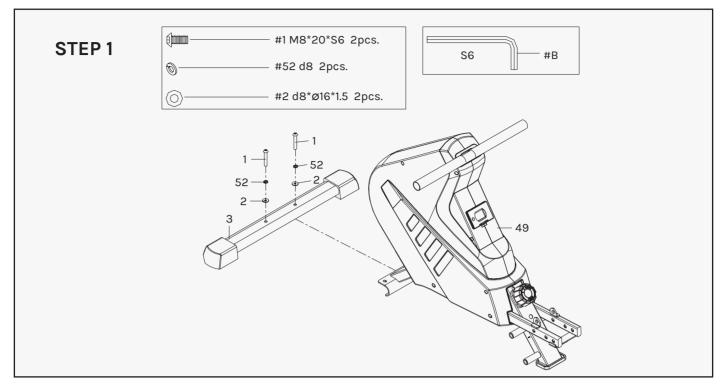
Attach Front Stabilizer (No. 3) to Main Frame (No. 49) using 2 Screws (No. 1), 2 Spring Washers (No. 52) and 2 Washers (No. 2). Tighten and secure with Allen Wrench (No. B).
