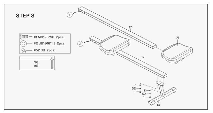
Insert Seat (No. 71) onto the Sliding Rail (No. 17).
