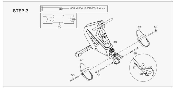
Attach 2 Bolts (No. 58) into the bottom hole of Main Frame (No. 49) with Spanner (No. C). Attach 2 Bolts (No. 58) through the Pedals (No. 57), into the upper hole of the Main Frame (No. 49), and tighten with Spanner (No. C).
