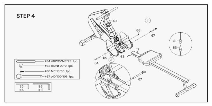
Connect Sliding Rail (No. 17) to Main Frame (No. 49) using Bolt (No. 64), Washer (No. 65) and Screw (No. 66). Tighten and secure with Allen Wrench (No. A) and Allen Wrench (No. B).
