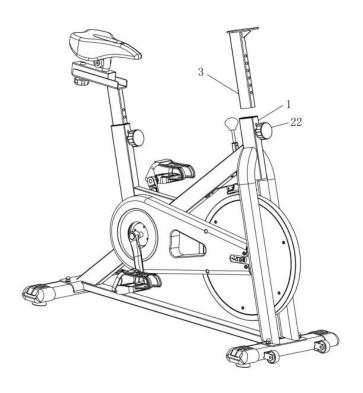
1. Loosen the adjustable knob (22) and insert the handlebar stem (3) into the mainframe (1). After align the hole to the adjustable knob (22), then secure the adjustable knob (22).
