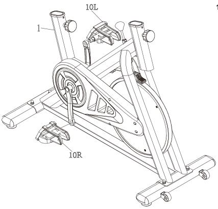
Screw the right pedal (10R) into the crank shaft in the CLOCKWISE direction.
