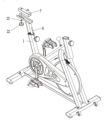
Put the seat slider (7) into the seat post (6). The bolt which is welded on the bar (7) must be located into the slot of the seat post (6). Then tighten it with fixing knob (22).
