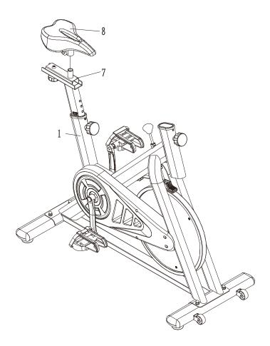
1. Slide the seat (8) onto the rod of the seat bar (7) .Then tighten the two nuts under the seat (8) securely.
