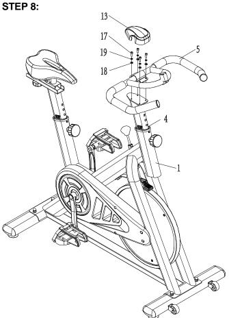
1. Put the handlebar (5) onto the handlebar stem (4) and make the holes aligned completely. Tighten them with 4 sets hexagon socket bolts (17), spring washers (19) and washers (18) securely.
