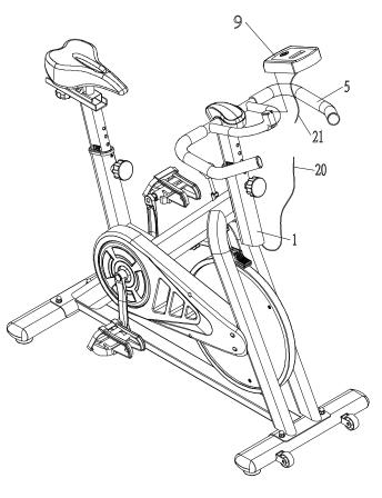
1. Secure the console (9) to the handlebar (5). Then connect the console cables (21) to Sensor Cable (20).
