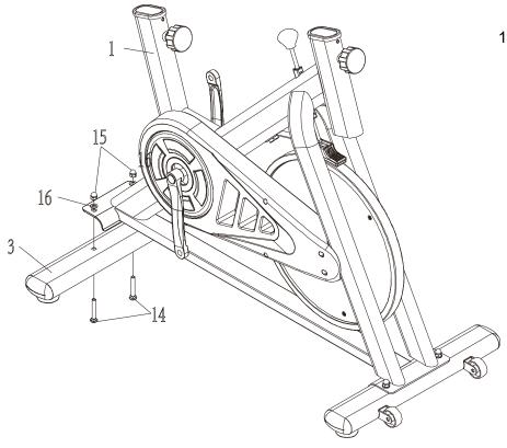
1. Secure the rear stabilizer (3) to the main frame (1), using 2 sets carriage bolts (14), dome nuts (15) and washers (16).
