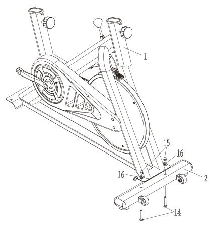
1. Secure the front stabilizer (2) to the main frame (1), using 2 sets carriage bolts (14), dome nuts (15) and washers (16).
