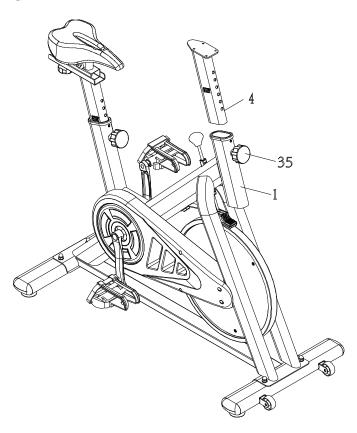
1. Loosen the adjustable knob (35) and insert the handlebar stem (4) into the mainframe (1). After align the hole to the adjustable knob (35), then secure the adjustable knob (35).
