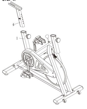
Loosen the adjustable knob (35) and insert seat post (6) into the main frame
