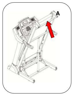
Place your hand on position (A), then pull up the base frame until you hear the click sound emitted when the air pressure bar (10) is locked into the round tube.
