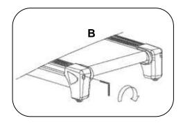
To adjust the **tightness** of the belt: turn both the left and right adjusting bolt 1/4 turn clockwise. Then start the treadmill until belt centers. Repeat until the belt correctly tightens. *Picture C*
