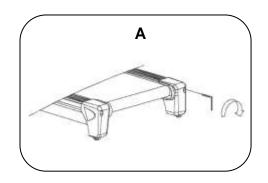
If the belt has drifted to the **left**: turn the right adjusting bolt 1/4 turn clockwise. Then start the treadmill until belt centers. Repeat until the belt correctly centers. *Picture B*
