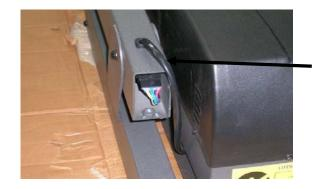
Pay special attention to the data cable when placing the right upright into its vertical position. Ensure computer cable is held tight to prevent damage. Any damage done to the cable will cause the machine not to function correctly and may not be covered under warranty.
