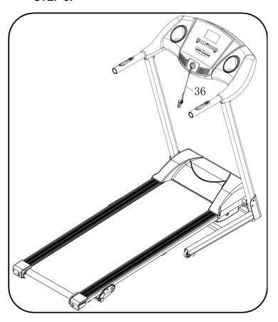
Place the safety key (36) into its dock on the display and switch the power switch on.
