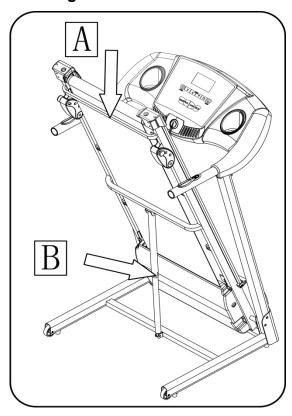
Place your hand on position (A), then pull up the base frame until you hear the click sound emitted when the air pressure bar (B) is locked into the round tube.
