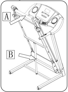
Whilst supporting position (A) with our hand, gently push position (B), the marked area on the air pressure bar, with your foot. The base frame will descend automatically. (Please keep people and any pets away the machine during descent)
