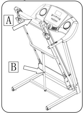
Whilst supporting position (A) with our hand, gently push position (B), the marked area on the air pressure bar, with your foot.
