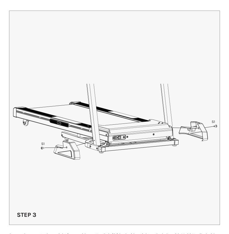
Secure the cover to the upright frame with one Hex Bolt (S1) both sides, tighten the bolts with Multi Hex Tool with Allen Key provided.
