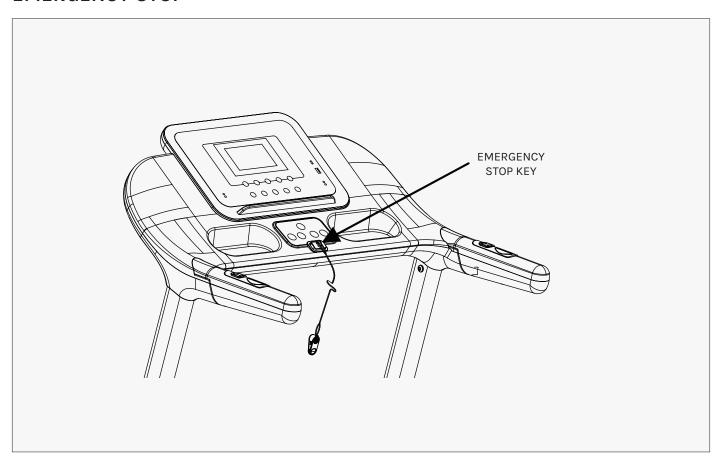
Before beginning a workout session ensure that the EMERGENCY STOP KEY is placed onto the Computer Console and the Safety Clip is securely attached to an article of your clothing. If you fall the clip will pull out the **EMERGENCY STOP KEY** from the Computer Console and the running belt will stop immediately for emergency stop, helping to prevent injury.
