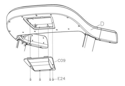
Disassemble the Console back cover (C09). Loosen 4 x screw (E24) and remove the Console back cover (C09) by using cross wrench with screw driver (B12).
