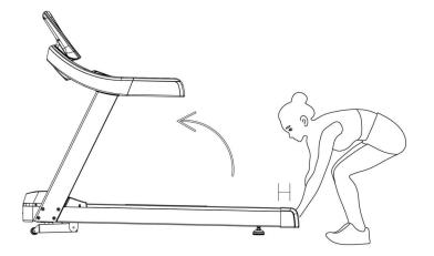
How to move the machine1. Hold the end of the machine (figure H) and tilt machine on its wheels.
