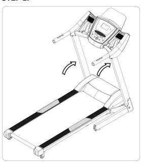
Raise the Computer and Upright tubes in the direction of the arrows.
