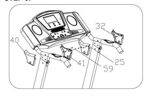
With ST4.2\*12 Screw (59), insert the UPRIGHT COVER (25, 32, 40, 41) onto the L&R handle bar.
