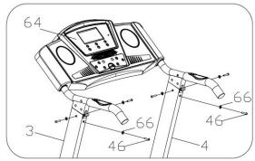
Use the 5# Allen wrench, screw through the bolt (46) to Lock washer (66), then lock the COMPUTER (64) onto R&L upright (3,4).
