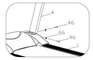
Using the 5# Allen wrench, screw through the bolt (46) to Lock washer(66), then lock the Right upright (4) onto MAIN FRAME (1)
