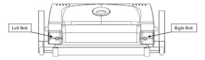
Note: Adjustment is through small hold of end cap.
