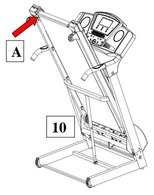
Support position A with your hand, then pull up the running board following the arrow direction until you hear a clicking sound of the cylinder (10) locking into the round tube.
