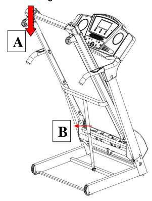
Support position A with your hand, depress position B of the air pressure control bar, then the base frame will descend automatically
