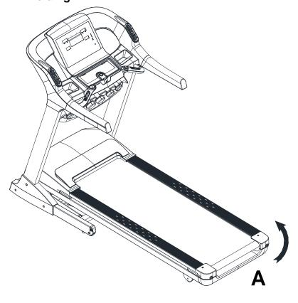
Place your hand on position (A), then pull up the base frame until you hear the click sound emitted when the air pressure bar (B) is locked into the round tube.
